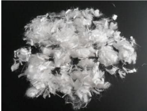
(a) Polypropylene fibers with 12mm length (b) SEM image of polypropylene fiber [28] Figure - 2
